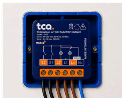
Figure 5: Raccordement du module
